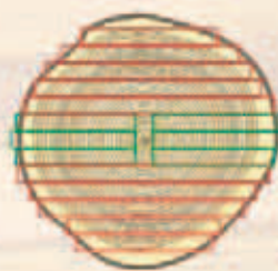
Tangential flat-sawn section
