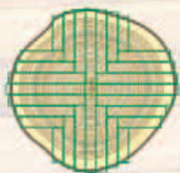
Comb-grained sawn section
